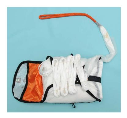
Insert the folded lines into the container and close it as shown in the pictures:
