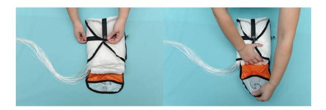
9. Finally, we come to the packing of the lines. We pack them manually or with the help of a special tool for line packing, as it is shown in our case. In any case it is important to match the width of the container on the side, where the pocket for inserting the folded lines is located, while stacking the lines.
