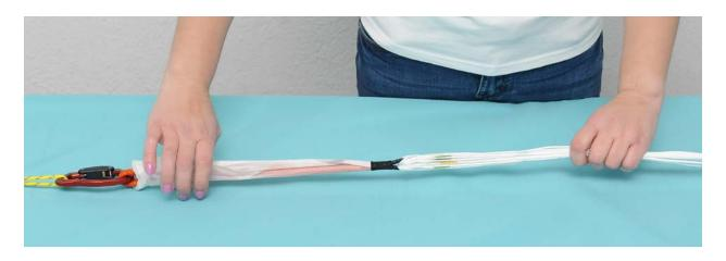
2. Find panel no.1, separate the panels and lines so that an equal amount lies on each side.
